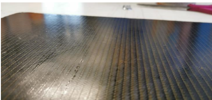
Image of a post-cured 3R resin infused plate
